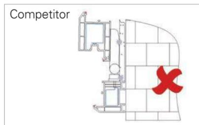
This hinge is too bulky for the frame, so there are two impact points on the internal plaster reveal.
