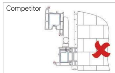
To overcome this, an add-on profile gives the hinge clearance – but this reduces the available clear opening width of the door and adds cost.
