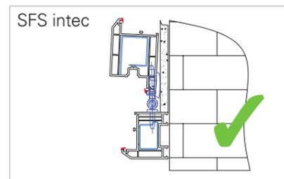
The obvious solution is the slimmer Dynamic 2D hinge which maximises the door opening width with ease.
